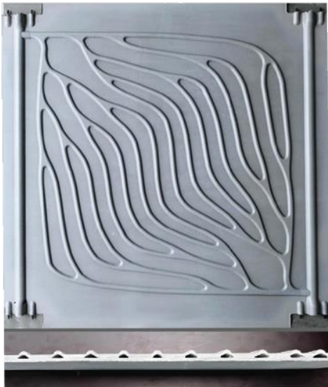
Rear side of a TABSOLAR® panel with bionic FracTherm® channel structure, side collection channels und hydraulic ports (above) and cross section of a TABSOLAR® panel (below). © G.tecz Engineering GmbH
