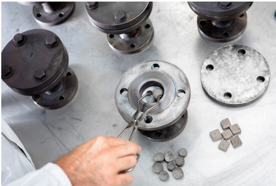
The compatibility of the filler materials and different high-temperature media was investigated by means of ageing tests. The different geometries are used to check the mechanical stability before and after the tests. ©Fraunhofer ISE
