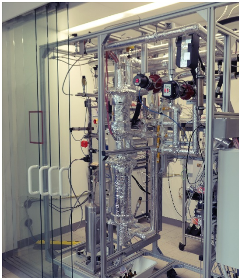
Methanol synthesis from metallurgical gases was successfully demonstrated in the miniplant. ©Fraunhofer ISE
