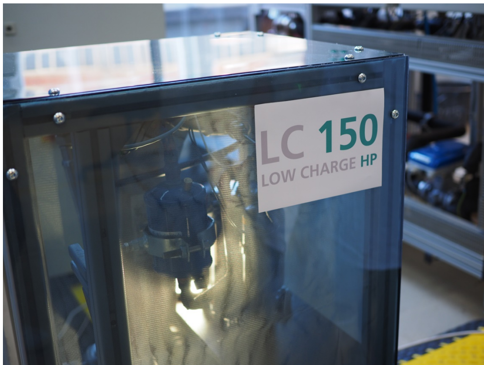
The LC 150 heat pump developed at Fraunhofer ISE is based on the climate-friendly refrigerant propane. ©Fraunhofer ISE
