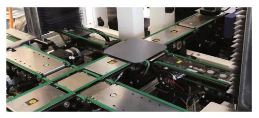
Inline characterization: Wafers are sorted using predefined algorithms or measurement results. ©Fraunhofer ISE
