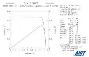
IV characteristics of the new 4-junction solar cell with an efficiency of 46% at 50.8 W/cm<sup>2</sup> which corresponds to a concentration ration of 508 times the solar AM1.5d (ASTM E927-10) spectrum.
