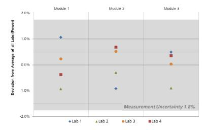
The round robin tests of the four internationally top calibration laboratories for PV modules all had measurements with deviations of  $\pm 1\%$  from the mean, and thus well within the measurement precision of 1.8% at the Callab PV Modules of Fraunhofer ISE ©Fraunhofer ISE
