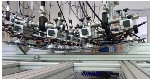
TPedge module passes mechanical load test. ©Fraunhofer ISE
