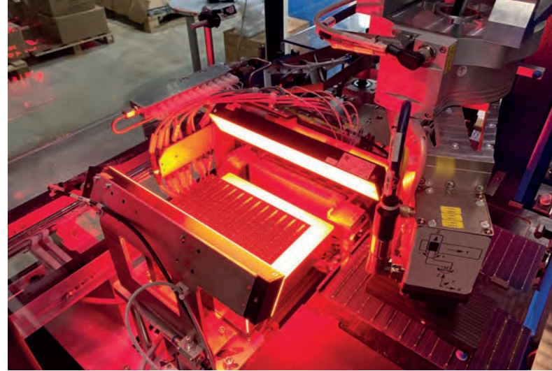
Solar cells on the breakage control unit of the stringer in the Module-TEC production laboratory of Fraunhofer ISE (G12 half cells)
