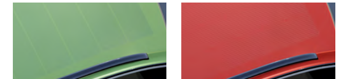
Visualisation of a car roof with (left) shingle technology and (right) wire interconnection technology.
