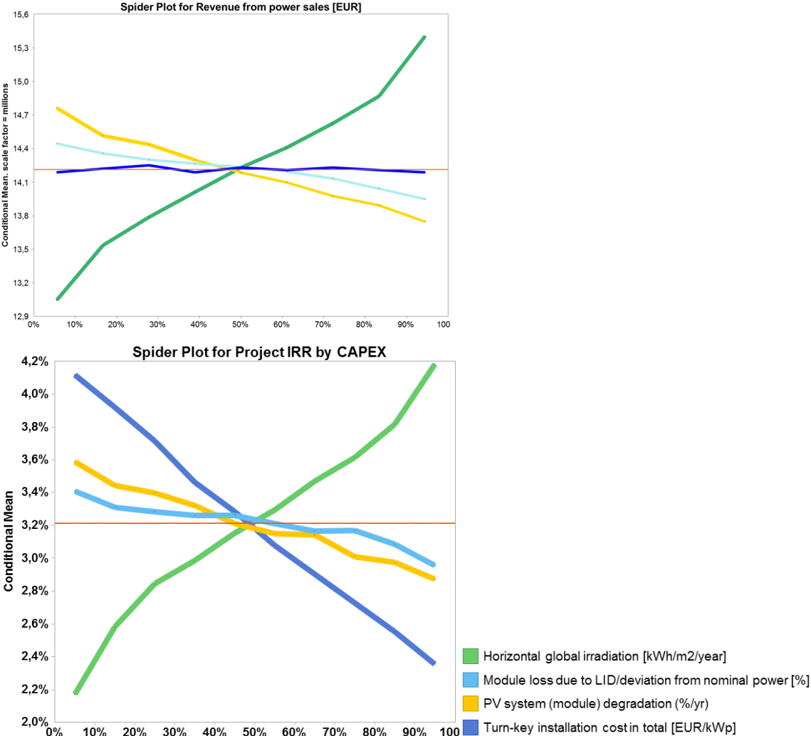
Figure 18: Spider plot demonstrates how the revenue from power sales measured in units of million EUR (top) and Project IRR by CAPEX as given by non-unit values (below) varies as a function of a percentage-wise change in the input variables that have been selected as object for investigation of being uncertain.
