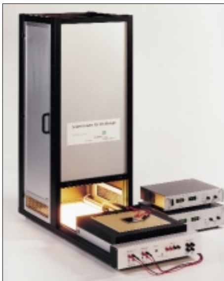
Fig. 1: Solar simulator to characterise CIS modules, developed and constructed for the Siemens Solar company, Munich.
