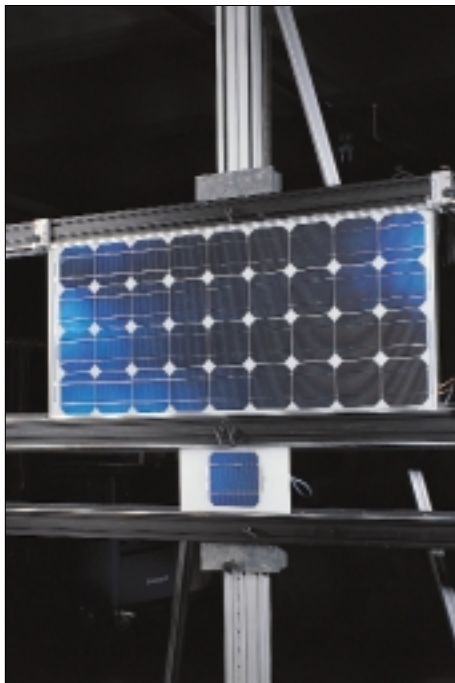
Fig. 1: Solar module and reference cell mounted for measurement with the pulsed solar simulator.
