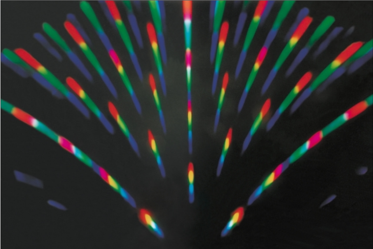
Dispersion of white light by diffraction with a periodic surface structure (optical grating). Large areas of periodic and stochastic structures are employed in anti-reflective, light-scattering, dirt-repellent and other functional surfaces.
