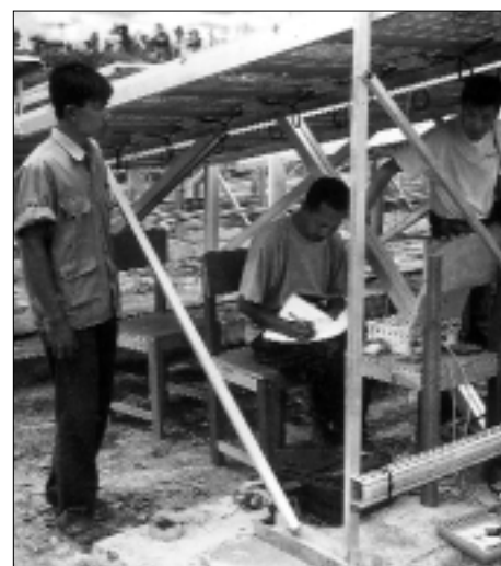
Fig. 1: Investigation of a technical system: The photo shows on-site measurement of photovoltaic strings in operation. The measurements are made by an Indonesian staff member.
