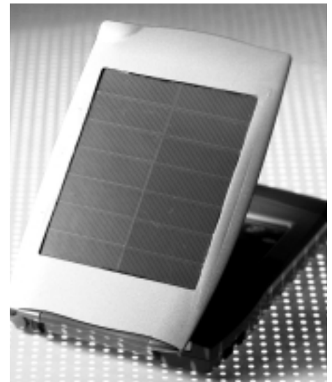
Fig. 1: Prototype of a solar-powered organiser. The rechargeable batteries, which are integrated into the device, are charged by the photovoltaic module. (Co-operation between Fraunhofer ISE, Casio Computer and AccuCell).
