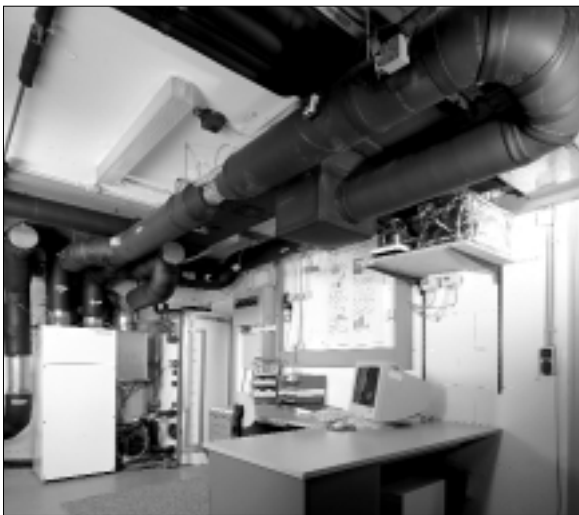
Fig. 1: Automated test stand with room for two separate ventilation devices with exhaust air heat pumps.
