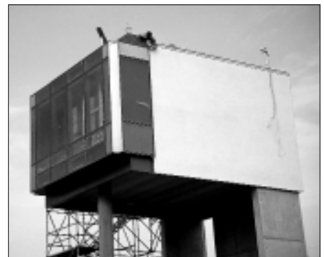
Fig. 6: Test cell from a high-rise building with a double envelope, for the new headquarters of the Fraunhofer Society in Munich.
