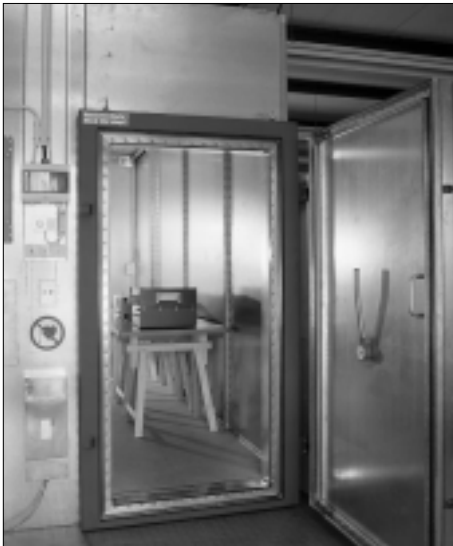
Fig. 1: View into the EMC measurement chamber at Fraunhofer ISE.
