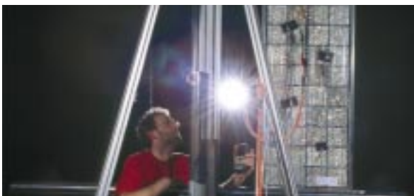
Fig. 2: Significant progress in the module calibration at Fraunhofer ISE was made by renewing the hardware and software of the measurement technology. Now that the homogeneity of the illumination has been improved significantly, the calibrated reference cells from the Physikalisch-Technische Bundesanstalt can be used directly for the module measurements. For standard measurements without correction for the spectral response, a measurement uncertainty of less than \pm 4\% is expected and for precision measurements, this is reduced to about \pm 2.5\% .
