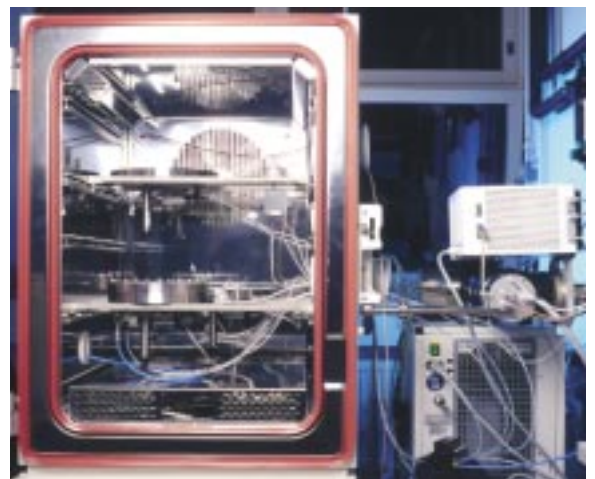
Fig. 3: Permeation measurement of high-barrier films using mass spectrometry. These films are used, for example, as the backing films for photovoltaic modules or for the envelope of vacuum insulation panels.
