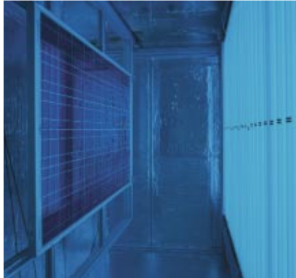
Fig. 1: UV test stand for photovoltaic modules with dimensions up to 1.4 x 2.4 m 2 : The intensity of the UV radiation is 50 times higher than the natural UV-B radiation and 7 times higher than the natural UV-A radiation.
