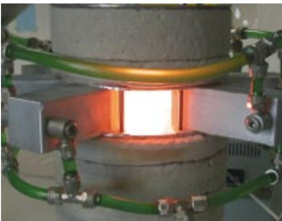
Fig. 1: TPV test generator operating at 1200 °C at Fraunhofer ISE. Eight GaSb modules, which are mounted on water-cooled supports, are located concentrically around the radiation emitter. One GaSb module and its cooling block have been removed to reveal the glowing radiation emitter. The aperture has an area of about 5 x 5 cm 2 .
