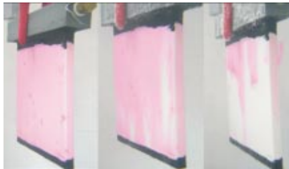
Fig. 2: A dyeing procedure is used to analyse the effect of different cleaning procedures optically. Here, the ultrasonic cleaning process with a frequency of 1 MHz is illustrated for a ceramic membrane plate with three images which were taken at intervals of 60 s. The dyed cover layers are loosened and swept away by the acoustic current, an ultrasonically excited motion of the fluid.
