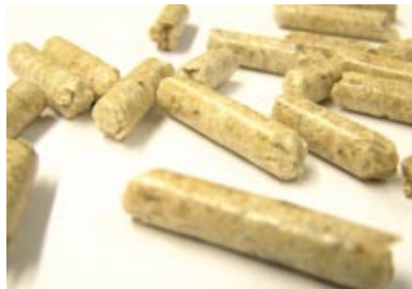
Fig. 2: Wood pellets are small cylindrical rods with a diameter of 6 to 8 mm and a length of 20 to 40 mm. They are made by pressing sawdust and other wood remnants. In contrast to fossil fuels, wood pellets are CO 2 neutral, because combustion only releases the amount of carbon dioxide which had previously been absorbed by the tree during its growth.
