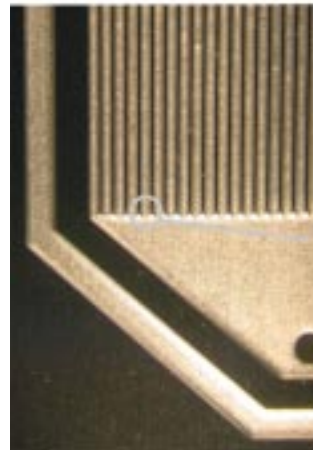
Fig. 4: Etched metal films with parallel channels, which are used as the anode gas distribution structure of a miniature fuel cell. The etching process allows extremely fine geometric structures to be produced, so that there is no need for a gas diffusion layer.
