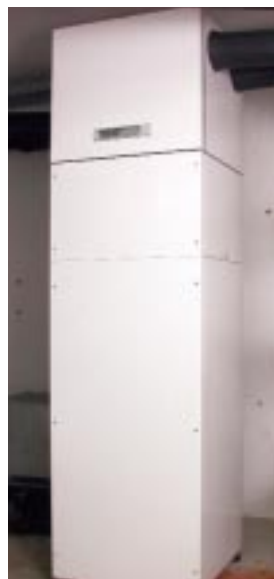
Fig. 3: Compact heating and ventilation unit during measurement with the test stand. The unit is specially designed for use in passive multi-storey buildings and has a small, integrated storage tank with a capacity of 240 litres.
