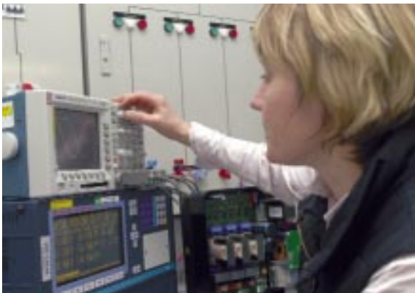
Fig. 2: The photo shows a high-precision power measurement instrument used for exact determination of inverter efficiency.
