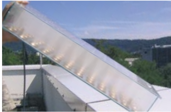
Fig. 2: Photo of a FLATCON® module. The light rays have been made visible here by injecting smoke into the module. The aperture area of a module is 768 cm 2 and is covered with 48 Fresnel lenses, each with an area of 16 cm 2 . A concentrator solar cell of III-V semiconductor material is located at the focus of each lens.
