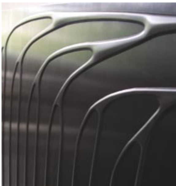
Fig. 2: Section of a solar absorber, with flow channels designed according to bionic principles with the FracTherm algorithm we have developed. The absorber is of aluminum and was made by the Alcan Rollbond company using the roll-bonding process.
