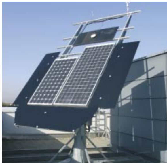
Fig. 2: Outdoor test stand to determine the "nominal operating cell temperature" (NOCT). The single-axis tracker allows the required testing times to be shortened.
