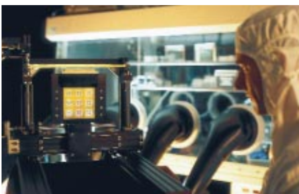
Fig. 2: Experimental equipment for automated measurement of the relevant solar cell parameters. The important measured characteristics include the solar cell characteristic I-V curve, the spectral response, the absorption, the linearity of the solar cell with respect to radiation intensity and the charge carrier mobility. With this equipment, the characteristic curves of 90 solar cells can be measured within an hour.
