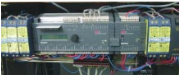
Fig. 1: This measurement data acquisition system is located in the village of Kesheng, 450 km away from Xining, the capital of Qinghai province. It records ten-minute averages of 15 measurement values. The data are transferred to Xining either via a telephone modem or with a replaceable memory card.
