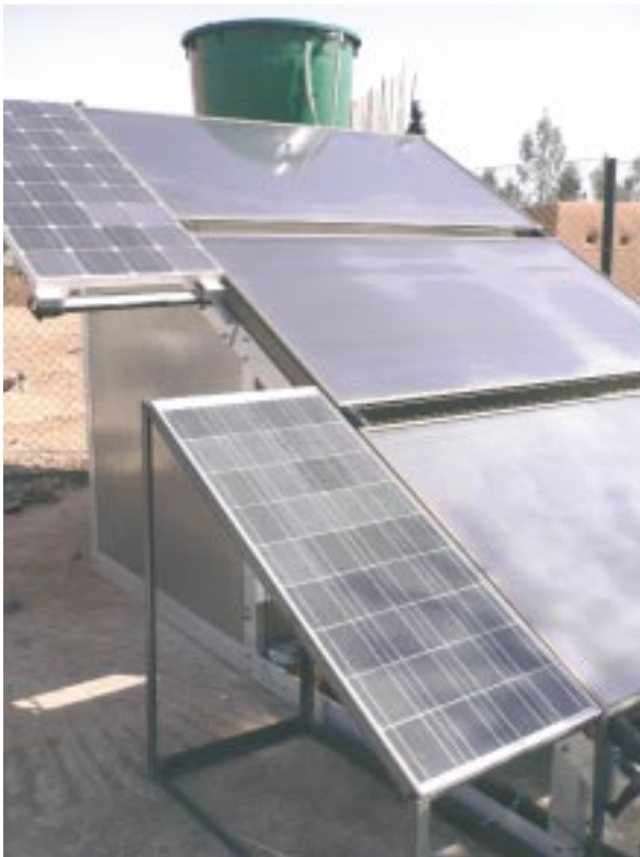
Fig. 1: The compact desalination systems developed at Fraunhofer ISE are operated solely by solar energy. As shown here in the Moroccan village of Kelaa, solar collectors with an area of 5.79 m 2 supply the thermal energy for membrane distillation and photovoltaic modules with a power of 106 W p (upper module) and 70 W p (lower module) supply the electricity to operate the pumps. The systems are thus completely independent of external sources of energy and can thus be operated in locations without a connection to the grid.
