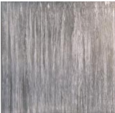
Fig. 1: Recrystallised wafer equivalent on a reaction-bonded silicon carbide ceramic substrate. The vertical, high-quality crystallites of the silicon layer, which are more than 10 cm long and up to 5 mm wide, are visible. The wafer equivalent in the photograph has an area of 180 x 180 mm 2 . The result shows that recrystallised wafer equivalents with excellent properties can be produced using production-relevant materials and processes.
