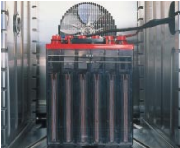
Fig. 1: In addition to efficiency and capacity, also the temperature dependence of properties such as the ageing and charging performance of storage batteries can be investigated. The photo shows the climatic chamber of the battery testing laboratory at Fraunhofer ISE.
