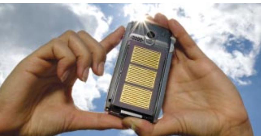
Fig. 1: Miniature fuel cells have the potential to lengthen the operating times of electronic devices considerably due to the increased energy storage density. Integration into mobile phones is seen as one of the most promising goals for miniaturisation.
