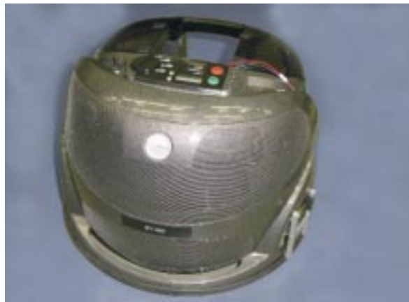
Fig. 3: The fuel cell system is being implemented in the commercially available vacuum-cleaning robot shown in the photo. A comprehensive navigation system maps the whole room and thus allows the load demand to be determined, which must be supplied by the fuel cell system. The vacuuming motor can be switched off while previously cleaned zones are traversed. A dust sensor is used to determine the power needed by the vacuuming motor.
