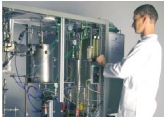
Fig. 1: Fully automated system for autothermal reforming of desulphurised kerosene Jet A-1 as the fuel for an SOFC (photo without SOFC). It is a system with integrated heating, i.e. the waste heat from the fuel cell is fed back to the reformer. The reformer system can be operated to track the fuel cell load, and can generate synthesis gas with a flow rate varying continuously between 10 and 45 NI per minute.
