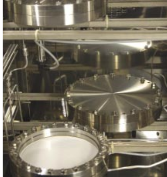
Fig. 1: Permeation measurement facility to determine the permeation coefficients of different gases and water vapour through films. The concentration of the gas to be tested is set on one side of the film. On the other side, a mass spectrometer measures the changing gas concentration in the sample holder (depth: 2 mm). The apparatus is located in a climatic chamber so that the temperature can be controlled.
