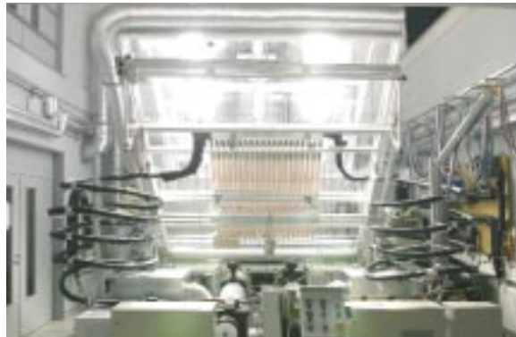
Fig. 1: Solar collector under the solar simulator of our indoor test stand during the stagnation measurement according to the procedure we have developed. To the left and right are the test pipes of the solar loop, with which the steam penetration distance can be measured. Temperature sensors, which are mounted along the test pipes at intervals of one metre, are used to measure whether the steam has reached a given position. From the known heat loss of the test pipes, it is possible to determine the thermal power which enters the solar loop piping in the form of steam and which must be dissipated by the piping to the surroundings.
