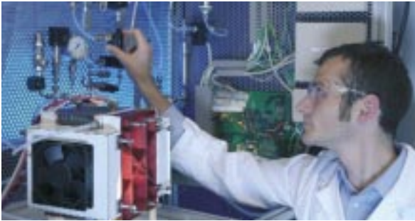
Fig. 1: Part of a system for long-term energy storage applying a reversible fuel cell. The fuel cell prototype from our project partner, the Energy Research Centre of the Netherlands (ECN), can be seen in the foreground. Fraunhofer ISE developed the complete system consisting of the cell stack, gas purification and storage, controls and voltage conversion.
