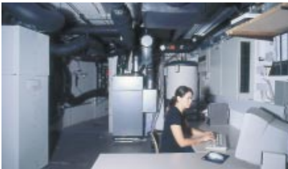
Fig. 1: In our test facility, we measure the energy efficiency of the complete units and their components. On the one hand, we can select from a wide range of stationary testing conditions. On the other hand, the automated controls allow us to apply dynamically changing conditions, e.g. according to the EN 255-3 standard. We derive recommendations for optimising the components and their interaction from the measurements.
