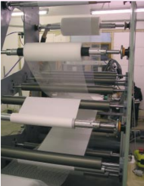
Fig. 1: The winding machine which was designed and constructed at Fraunhofer ISE to produce prototypes of spiral-wound modules for membrane distillation.
