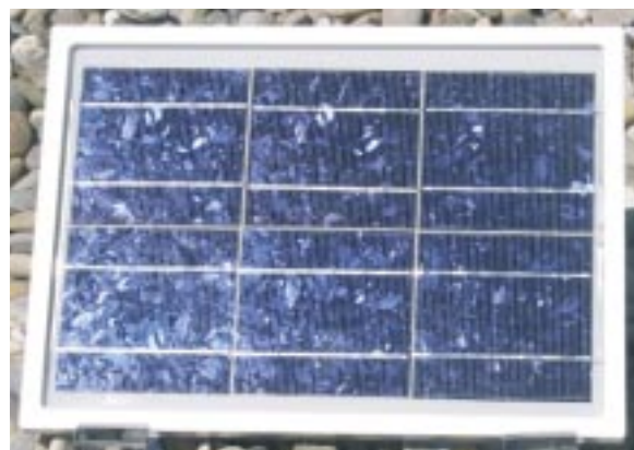
Fig. 5: A mini-module consisting of six multi-crystalline epitaxially prepared wafer equivalents of area 10 x 10 cm 2 . Although it was processed and looks like a "normal" module, it is really a genuine thin-film module.
