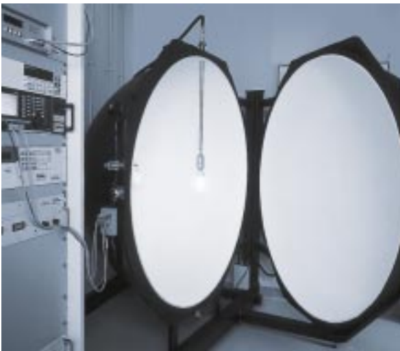
Fig. 2: Integrating-sphere photometer to measure the luminous flux of DC lamps and light sources.
