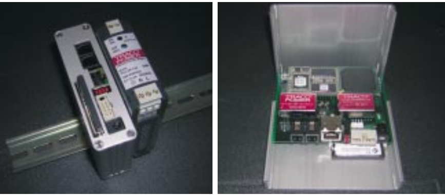
Fig. 2: The dialogue between the central energy management system and the components is maintained via the "PoMS Interface Boxes" developed at Fraunhofer ISE. They interpret commands from the central management unit and produce generation predictions for certain component types, such as photovoltaic systems.
