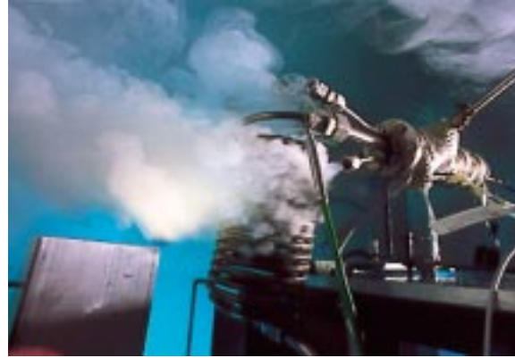
Fig. 1: New vaporiser in operation: "gaseous" diesel is visible as the white "clouds" leaving the opened outlet.
