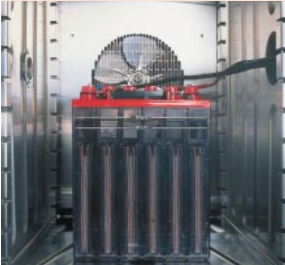
Fig. 1: In addition to efficiency and capacity, also the temperature dependence of properties such as the ageing and charging performance of storage batteries can be investigated. The photo shows the climatic chamber of the battery testing laboratory at Fraunhofer ISE.
