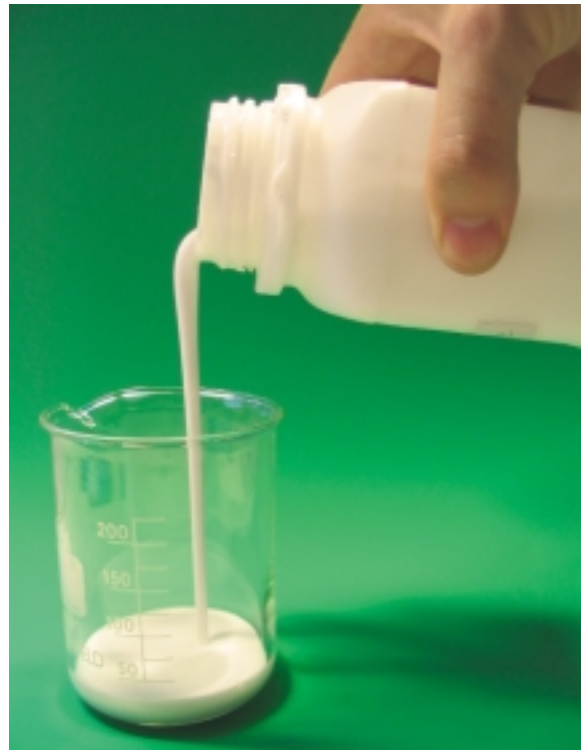
Fig. 1: PCS are fluids which can store very large amounts of heat with small temperature differences. They consist of a carrier fluid and a PCM additive. Appropriate measures ensure that the mixture remains liquid even when the PCM has solidified.
