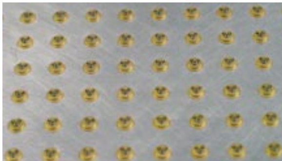
Fig. 4: Photo of laser power cells mounted on transistor housings. The cells convert light to electricity with an efficiency value exceeding 45 %.
