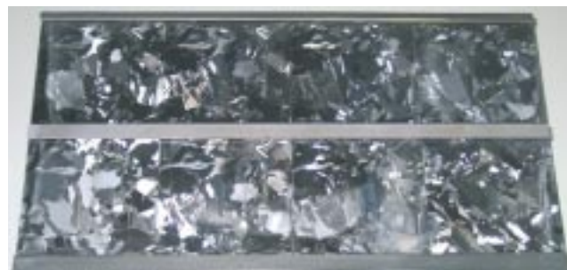
Fig. 4: A carrier loaded with test wafers of multi-crystalline silicon after epitaxial deposition of silicon. Depending on the crystal orientation in the substrate, the corresponding crystallites in the film grow at different rates, and differ clearly in their reflectance. The carrier dimensions are approximately 40 x 20 cm 2 .
