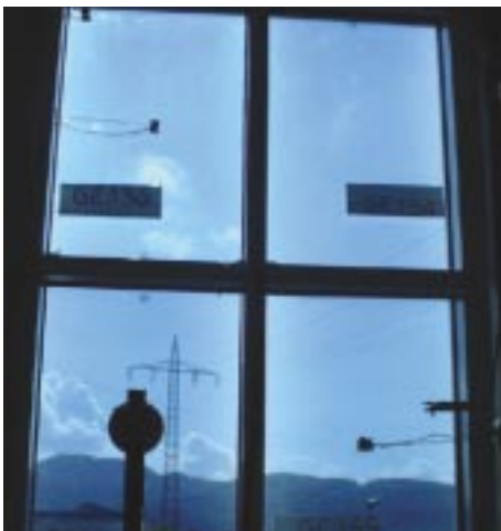
Fig. 1: View through gaschromic glazing with temperature and radiation sensors, in the facade test facility.
