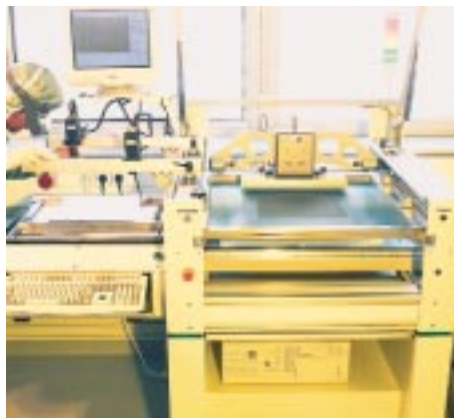
Fig. 1: Production technology for dye solar cells: All layers of the cell are applied by screen-printing.
