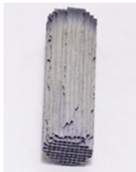
Fig. 3: Ceramic honeycomb to hold catalysts for screening tests for reforming liquid hydrocarbons.
