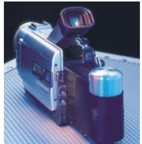
Fig. 3: Completely integrated fuel-cell system for a commercially available DV camcorder. Demonstration system developed by the Fraunhofer Initiative on Miniature Fuel Cells, under the leadership of Fraunhofer ISE.
