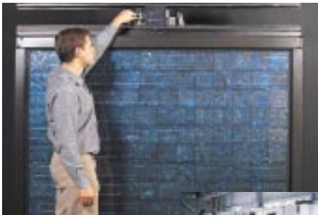
Precision measurement of a 3 m 2 solar module (article on p. 84).
