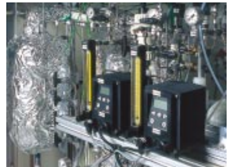
Fig. 1: Test stand for the POA kerosene reformer. The photo shows the educt inlets and the reactor.
