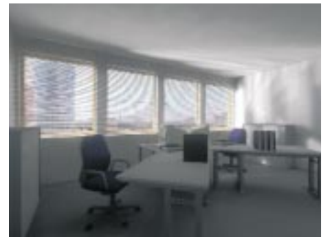
Fig. 4: Visualisation as the result of a lighting simulation calculation with a reflective blind slat.
