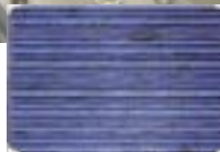
Epitaxial wafer equivalent on a highly doped silicon wafer, resulting in a cell efficiency value of 13.2 % (article on p. 39).
