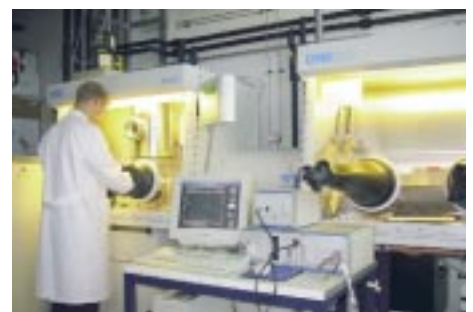
Fig. 3: Production of organic solar cells in the glovebox.
