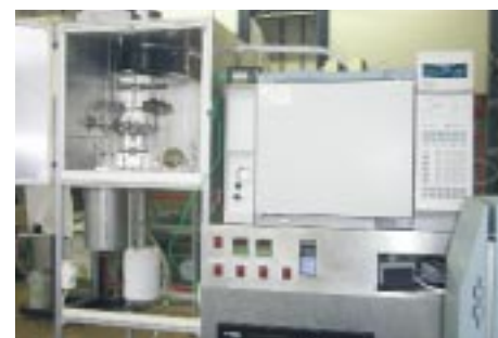
Fig. 4: Test stand to characterise catalysts for gas-processing technology. The gas chromatography equipment to the right of the photo is used to measure the composition of product and educt gases.
