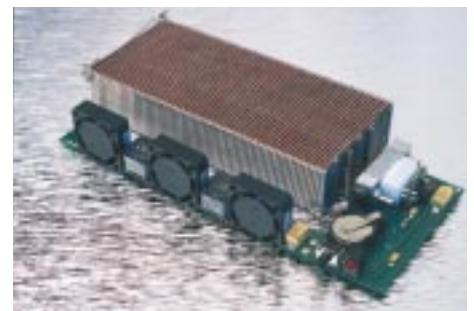
Fig. 4: 50 W fuel cell with a controls circuit board as a stand-alone power supply for a notebook.
