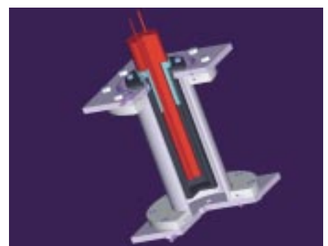
Fig. 4: 50 W fuel cell with a controls circuit board as a stand-alone power supply for a notebook.
