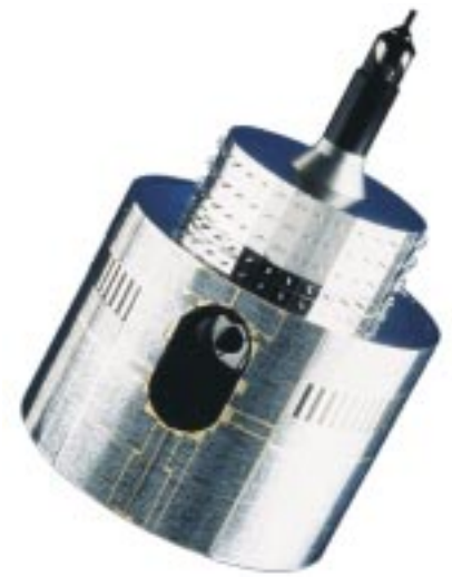
Fig. 1: METEOSAT 7 is the currently active, European geostationary meteorological satellite. Solar radiation maps with a resolution of about 5 \times 5 \text{ km}^2 in Central Europe are generated from its image data.
