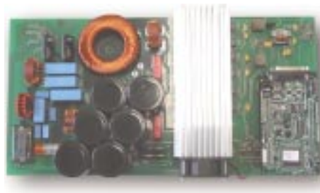
Fig. 1: Platform for inverters of the next generation, developed at Fraunhofer ISE. It uses the HERIC® topology.
