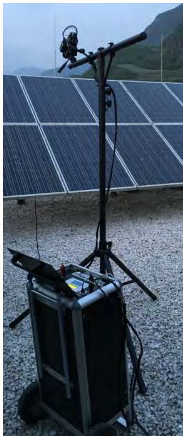
Figure 3-6: GreatEyes LumiSolar outdoor measurement system for field tests of PV modules.
