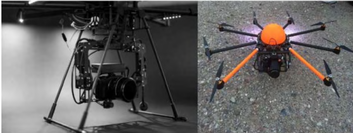
Figure 3-7: EL camera mounted on octocopter [79].
