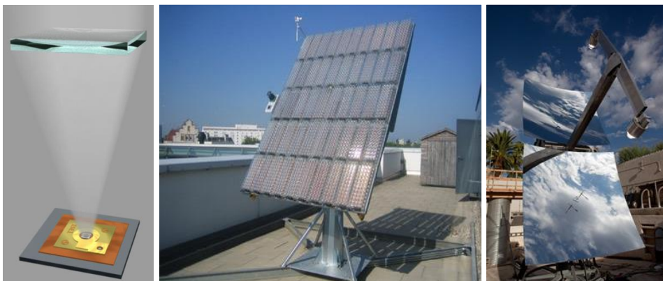
Figure 1: Left and middle: Example of a CPV system using Fresnel lenses to concentrate the sunlight: FLATCON ® concept originally developed at Fraunhofer ISE. Right: Example of a mirror-based system developed by the University of Arizona, USA [10].
