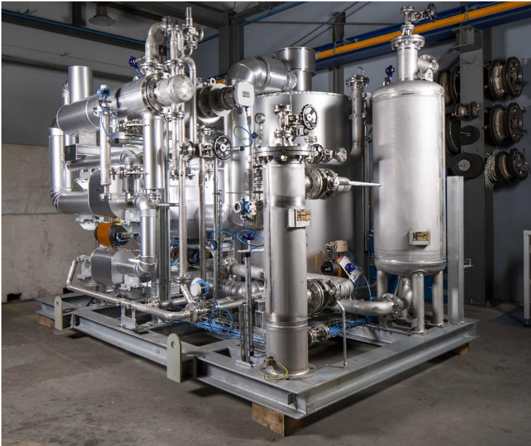
Figure 2-18: Gas purification system for a capacity of 4,000 Nm 3 /h (~20 MW electrolysis) (courtesy of Silica Verfahrenstechnik GmbH)
