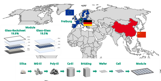
Figure 1: World map depicting the production location China (red), Germany (blue with green stripes) and the EU as of 2020 (blue) and the installation site in Freiburg, Germany, including the representation of the entire value chain (bottom) and the investigated glass-backsheet and glass-glass module designs with the corresponding efficiency (left).
