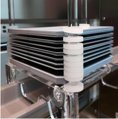
Figure 5: Experimental set-up for the stack oxidation process using a horizontal industrial tube furnace. Different groups of horizontally stacked wafers in this quartz boat are separated by quartz rings.
