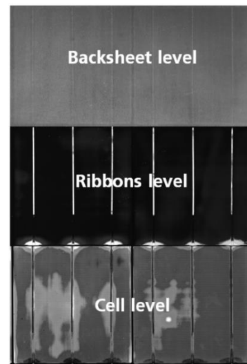
Figure 3 Acoustic micrographs (SAM images) generated from the different spectral regions ("gates") from a full-size module.
