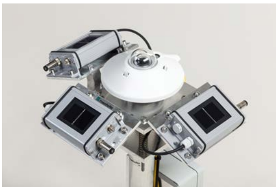
Figure 2: Measurement stations with a pyranometer to measure global horizontal irradiance and three silicon cells to measure global tilted irradiance, oriented towards east, south and west direction with 25° tilt angles.
