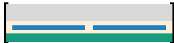
Figure 1: Simplified cross-section through a 4-cell mini module (not scaled). Shown components: frame (black), front glass (grey), encapsulant (peach), cells (blue), back sheet (green)
