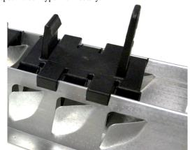
Figure 2: Detailed view of one cooling fin with the specially designed clamps.
