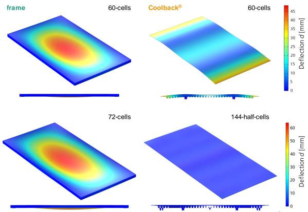
**Figure 4:** Simulated deflection at 2400 Pa push load in isometric and side view. Left: Conventional frame, right: Coolback® cooling fins, top: 60 cells, bottom: 72 cells / 144 half-cells. Please note, that in the Coolback® configuration for 60 cells four clamps and for 144 half-cells ten clamps are used.
