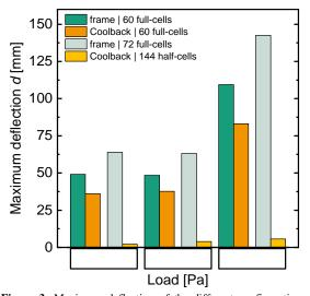
**Figure 3:** Maximum deflection of the different configurations for all simulated loads. Note: in the Coolback® configuration, four clamps are used for 60-cells and ten clamps are used for 144-half-cells.
