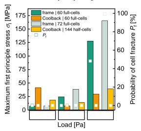
**Figure 5:** Maximum first principal stress  $\sigma_I$  (left axis) with the corresponding probability of cell fracture  $P_f$  (right axis) for all configurations and loads. Note: in the Coolback® configuration, four clamps are used for 60 cells and ten clamps are used for 144 half-cells.
