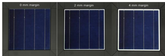
Figure 8: Layout of the apertures (masks) to measure the coupling gain for a specific margin where the backsheet
