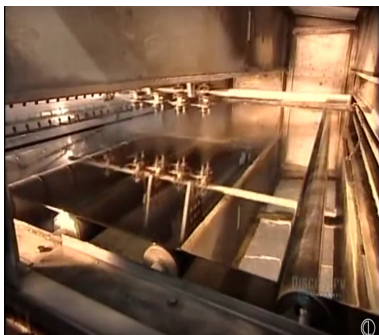
Fig 1: Photo of industrial Ag mirror production by spray deposition [2].
