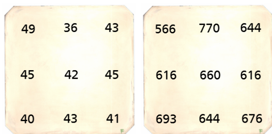
Fig. 7: Left: Photo of a 6 inch CZ Si wafer (without ITO in this case) chemically coated with Ag showing the measured sheet resistance of the deposited Ag in m\Omega/sq . Right: The same photo showing the thickness map of the Ag layer in nm calculated from the measured sheet resistance.
