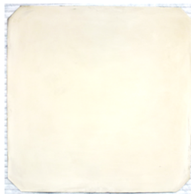
Fig. 6: Photo of a 6 inch alkaline textured CZ Si wafer (without ITO on the Si and without polymer ink at the edge) chemically coated with Ag.
