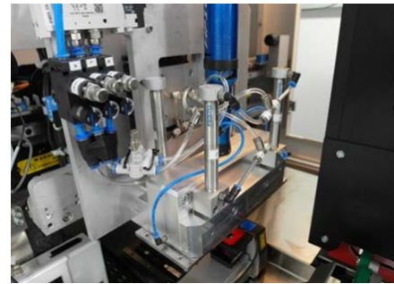
Figure 8: “Full wafer size” multi-nozzle dispense print head developed by Fraunhofer ISE and integrated in ASYS platform allowing for high printing speeds
