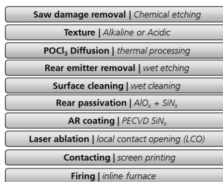
Figure 2 Process flow used for the fabrication of the PERC solar cells.
