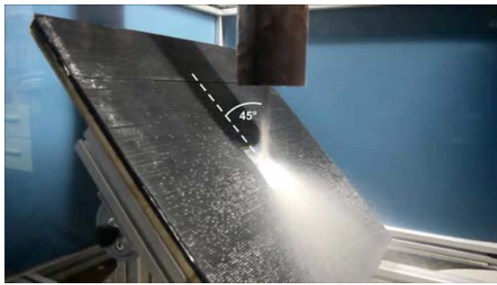
Figure 2: Focused sand stream at an impact angle of 45°
