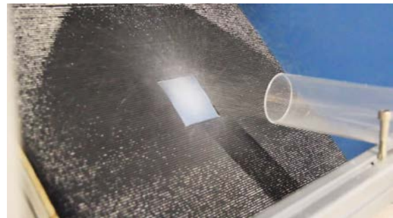
Figure 7: Sand blasting method on a reflector ( \alpha = 45^\circ )
