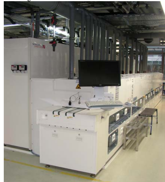
Figure 4: LINEA II is a fully automated wet chemical inline machine designed for the mass production of solar cells. The modular design of the process stations makes it possible to adapt the tool setup individually to particular cell concepts. Besides the proven wet chemical process steps like texturing, PSG removal and cleaning, the machine is also suitable for advanced inline processes like rear-side chemical polishing for PERC cells and chemical edge isolation.
