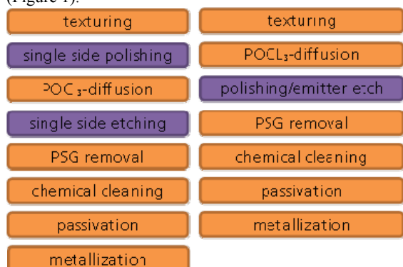
Figure 1: Process scheme for the PERC solar cell concept with the standard process (left) and combined
